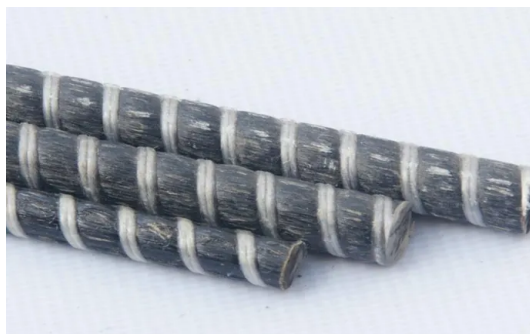
Fig. 5 · The helical fiber wrap over the basalt core (supplier photograph).
